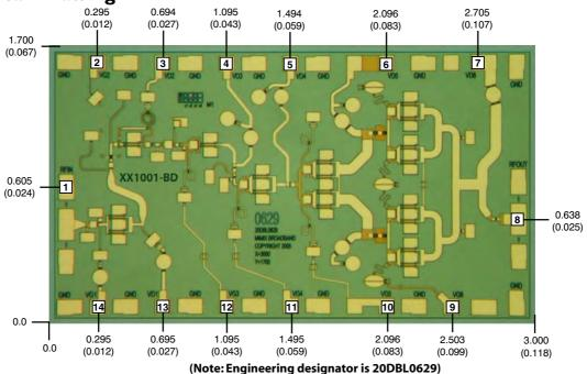
Units: millimeters (inches) Bond pad dimensions are shown to center of bond pad. Thickness: 0.110 +/- 0.010 (0.0043 +/- 0.0004), Backside is ground, Bond Pad/Backside Metallization: Gold All DC Bond Pads are 0.100 x 0.100 (0.004 x 0.004). All RF Bond Pads are 0.100 x 0.200 (0.004 x 0.008) Bond pad centers are approximately 0.109 (0.004) from the edge of the chip. Dicing tolerance: +/- 0.005 (+/- 0.0002). Approximate weight: 3.987 mg.
